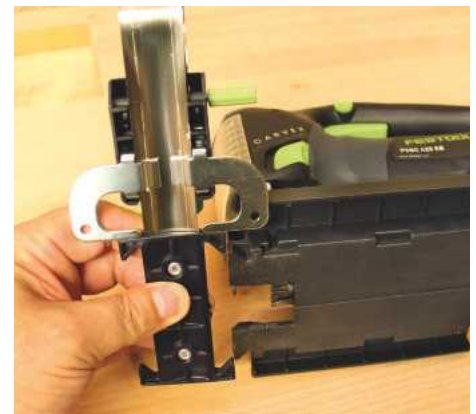
▲ This base doubles up as the circle-cutting guide or it will fit to a guide rail
